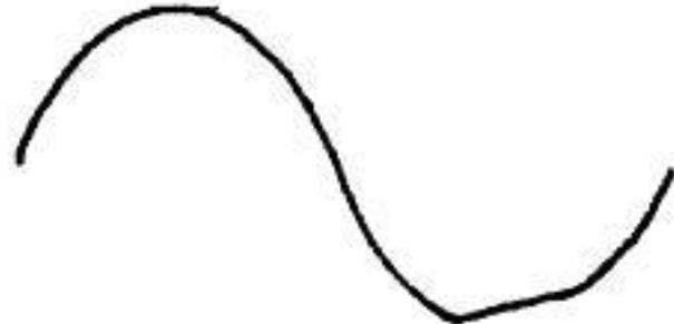
A Twin T oscillator slightly distorted, because it is tuned 5% higher than its initial frequency of oscillation. Its stability is excellent. It's dynamite for boxing.
